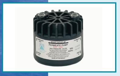
Aquatec's original Permeate Pump (ERP1000) is a simple, yet revolutionary, device. Powered only by the hydraulic energy of brine water usually lost to the drain (i.e. no electricity required), the Permeate Pump forces product water into the storage tank, reducing membrane back pressure and maximizing available feed pressure. These pumps dramatically improve the efficiency of R.O. water production, reducing wastewater by up to 80%. In other words, if your current system requires 10 gallons of tap
